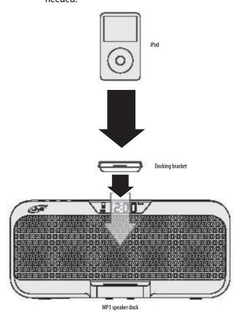
2 Snap the bracket into place over the iPod connector in the speaker dock.
